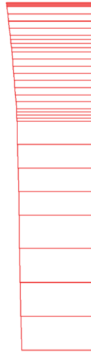
Fig. 129 Vertical displacements in beam (plate no: 1) Extreme value -247,11 \cdot 10^{-6} m (phase: 5)
