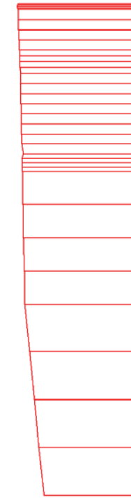
Fig. 28 Vertical displacements in beam (plate no: 2) Extreme value -52,38 \cdot 10^{-3} m (phase: 1)
